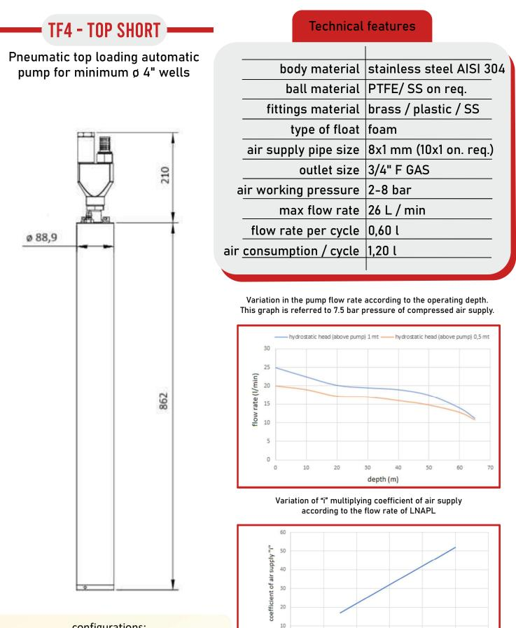
configurations: TF4-TOP SHORT (automatic) TF4-TOP SHORT T (timer + control panel) TF4-TOP SHORT HT (automatic for high temp.)
