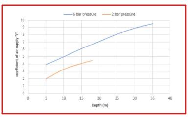
Variation in the pump flow rate according to the operation depth. This graph is referred to 2 m hydrostatic head and 6 bar pressure of compressed air supply
